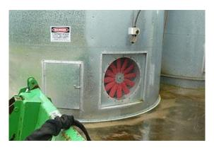
Holes in silo walls can allow air to escape leading to uneven drying of nut-in-shell and variable kernel moisture content.
